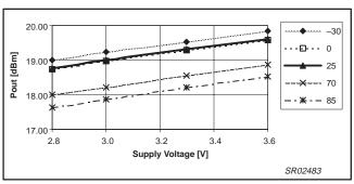
Figure 22. Output power vs. supply voltage, mode = high
